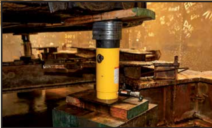
Hydraulic jacks used to lift USS Monitor 's turret.
