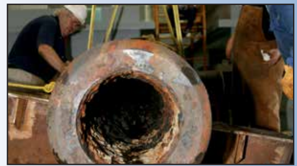
XI-inch Dahlgren shell gun from USS Monitor , showing marine corrosion in the bore. A specialized drilling platform must be designed and built to remove this material.
