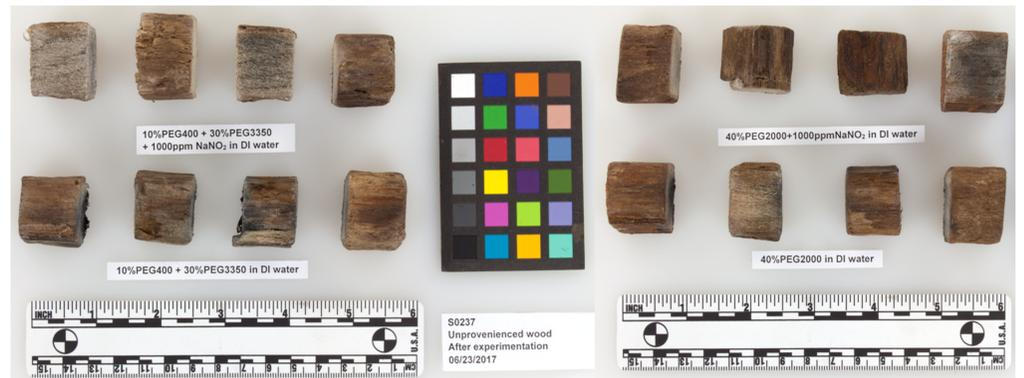
Figure 1: Wooden samples treated with 10% PEG 400 + 30% PEG 4000 with and without  $\text{NaNO}_2$ , and 40% PEG 2000 with and without  $\text{NaNO}_2$ .
