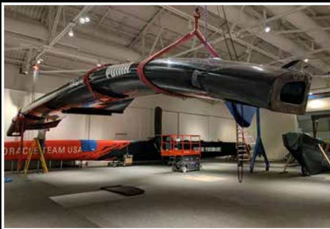
The two hulls of the catamaran, measuring 72 feet long, were shipped to the Museum separately from the crossbeam shown here, which measures 46 feet wide.
